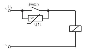
Example: Contact protection via a voltage dependent resistance (VDR)
