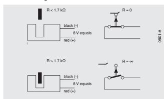
The control unit works, practically, without any reaction on the measuring system. The non-contact "contact system" produces no wear within the electrical system. The installed dimensions correspond to those of the model 821 contacts. The setting of the setpoints is made in the same way as for those contacts.
