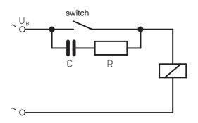
**Example: Contact protection via an RC-circuit**
