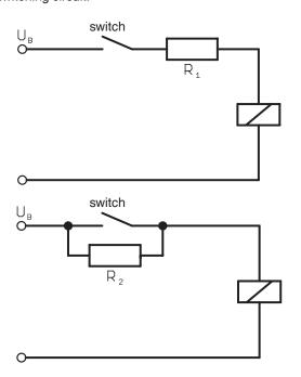
Example: Contact protection via a current-limiting resistance
